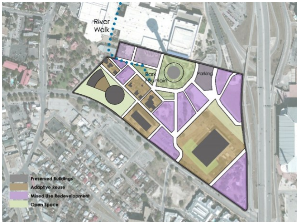
Figure 14 Design of concept two. The orange areas are the adaptive reused blocks that contain the preserved buildings. New mixed-use infill is marked in pink. Source: Christine Ma, group member
